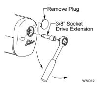
3. Turn the handle counterclockwise until the awning is retracted.
